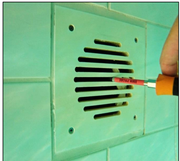
Photo 29: Wall inlets passed probe test
