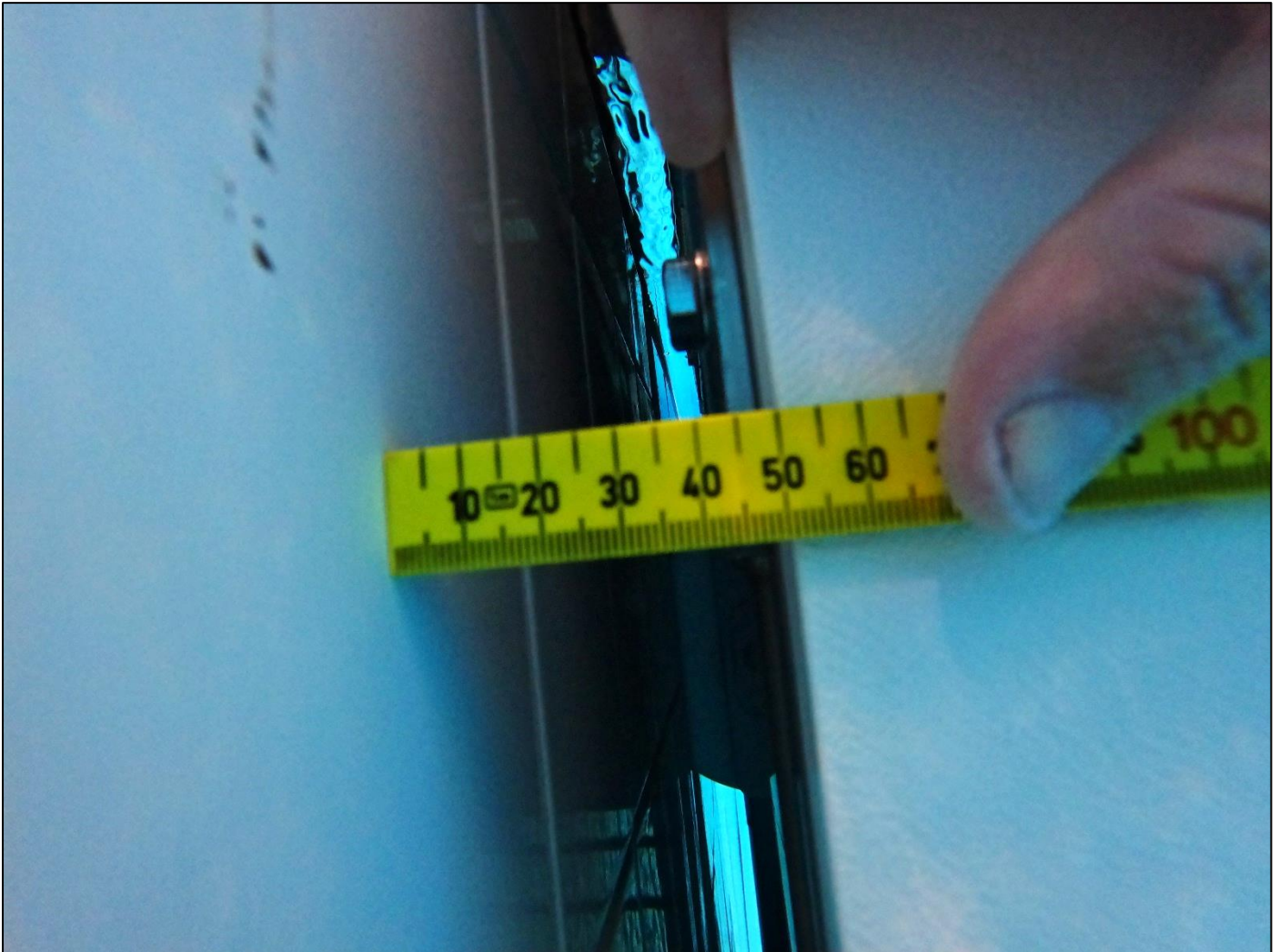
Photo 17: 50mm gap between pool wall and boom at 8 locations (Every corner of the 2 booms)
